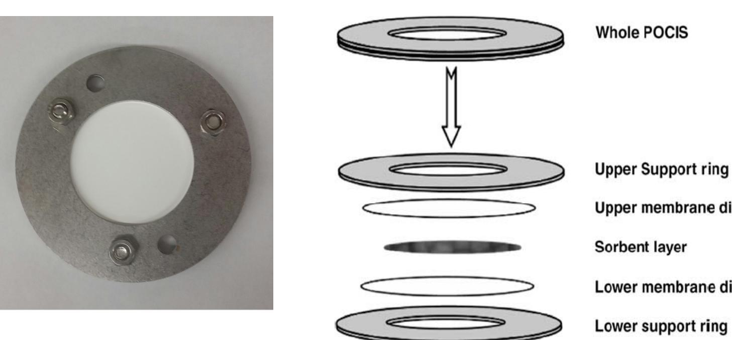
POCIS (Alvarez et al. 2010) sample weakly hydrophobic ( $\log K_{ow}$  up to 4) organic contaminants following strong binding to a polymeric sorbent (hydrophilic-lipophilic-balanced; HLB).
