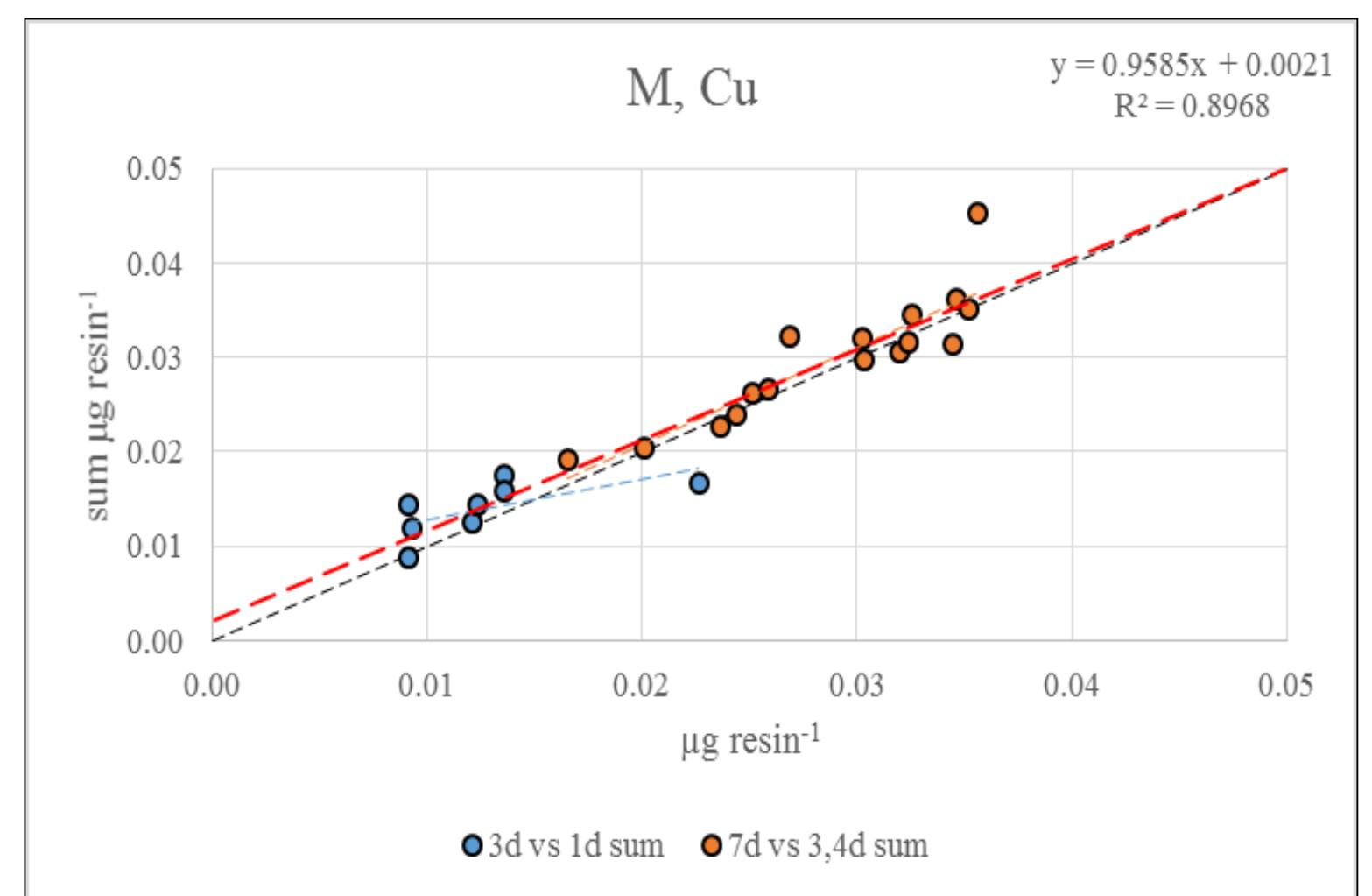
Cu mass accumulated on DGTs over 1, 3, 4, & 7 days shows linear uptake over time in seawater field deployments. The mass can be converted to the time weighted average of labile metals in the system by factoring the diffusional properties, area, and deployment time.
