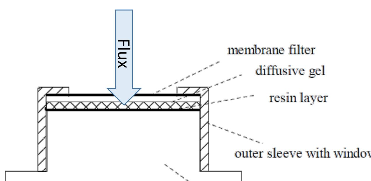
DGTs provide a time-averaged concentration of labile (biologically available) metal concentrations following diffusion through a gel layer and permanent binding to a resin layer (Chelex-100) (Davison and Zhang 2012).
