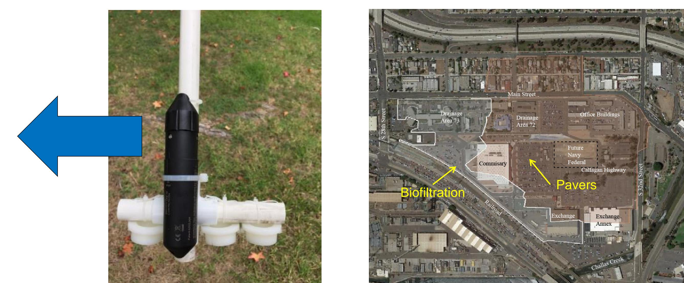
Application of a unique DGT approach for real time monitoring of metals in storm drains (above left) in short term ( $\leq 24$  h) exposures at two impervious sites at Naval Base San Diego (leveraged with NESDI #497) with focus on drains sampled before and after BMP treatment (above right).
