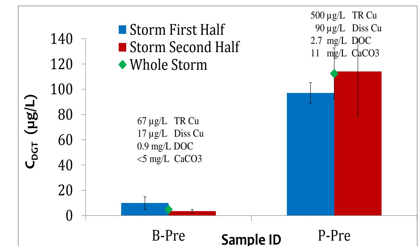
Comparison of first half and second half of ~24 hr storm in comparison with DGT samplers placed for full storm into freshwater drains. The 'B-Pre' and 'P-Pre' sample IDs represent untreated stormwater (prior to BMP treatment) the Biofiltration and Paver sites shown in photographs (at right).
