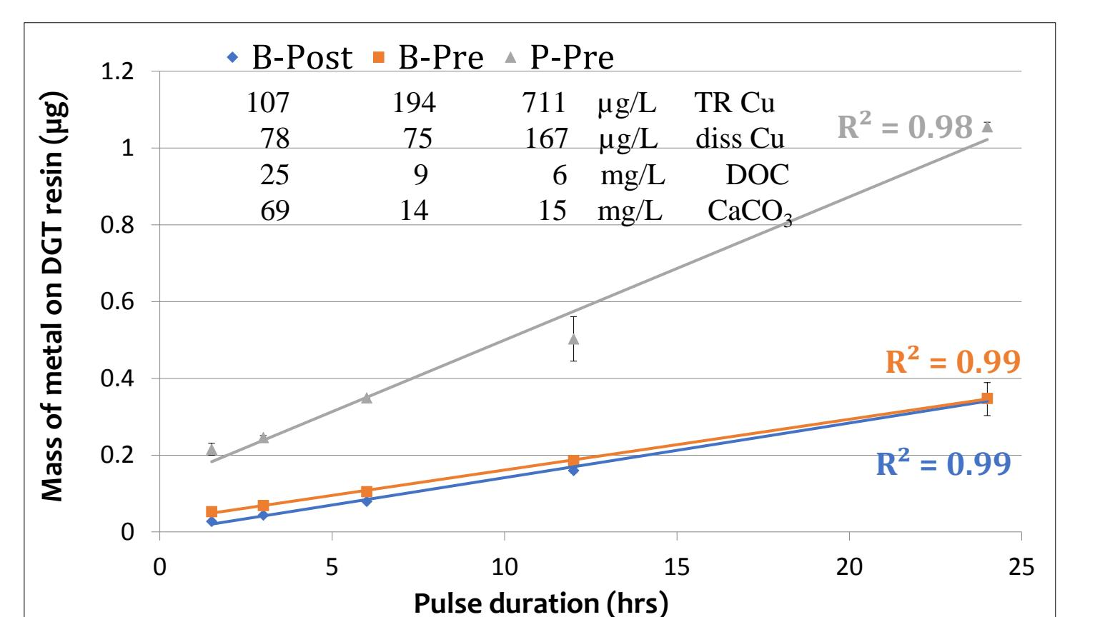
Linear loading of copper on to DGT Chelex-100 resin between 1.5-24 h durations in copper solutions. Shows detectable metal loading during short pulses.
